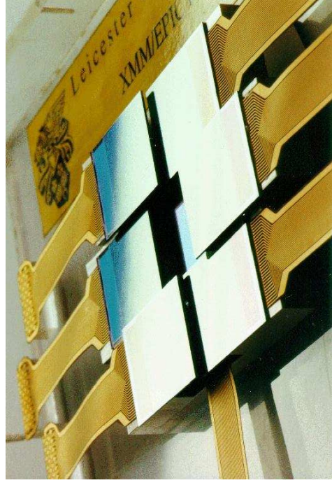
XMM-Newton (EPIC-MOS; Leicester): 7 single CCDs with 600 \times 600 pixels, mounting is adapted to curved focal plane of the Wolter telescope.
