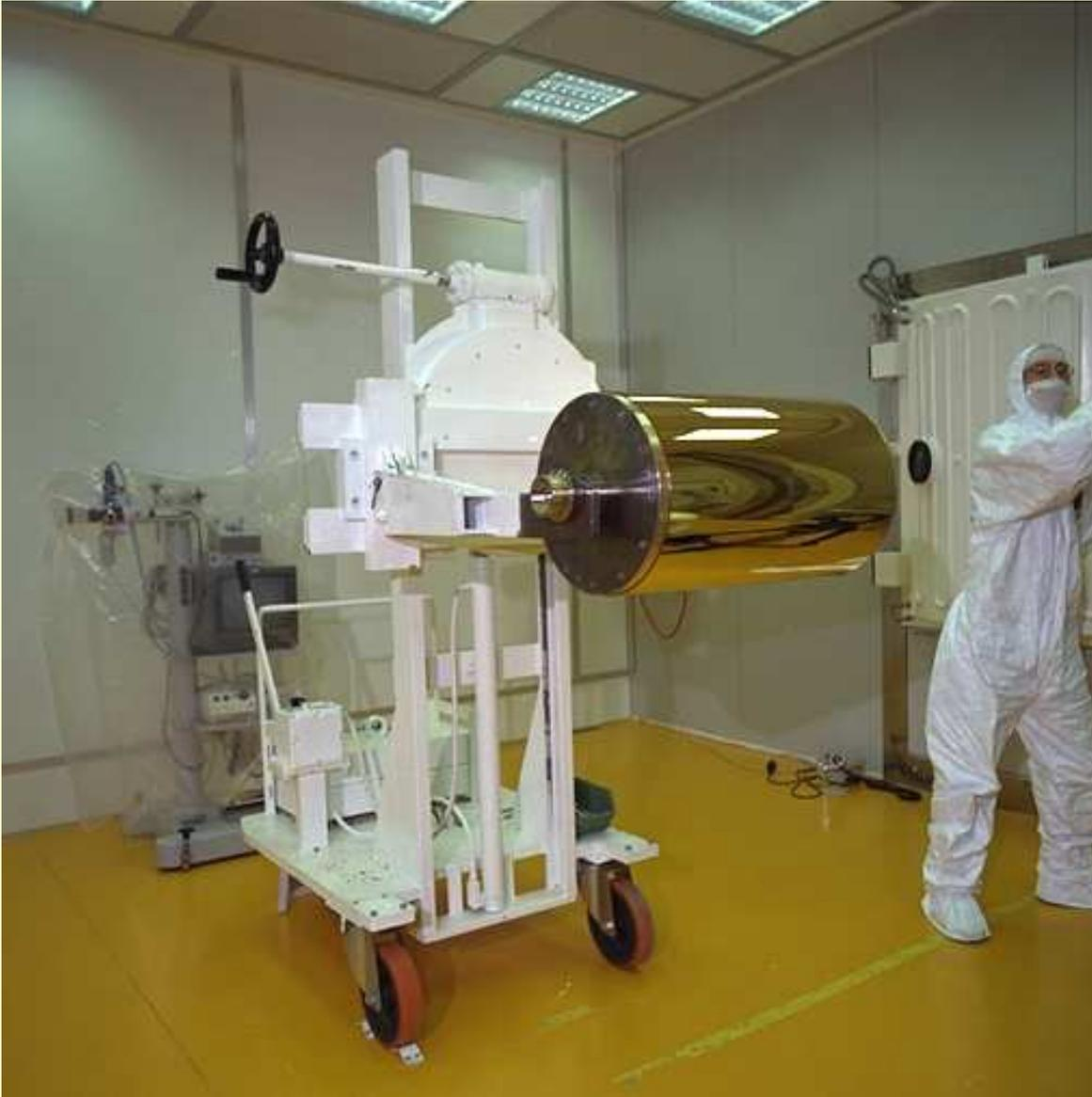
Gold plastered mandrel for one of the XMM mirrors before electroforming the Ni shell onto the gold.
