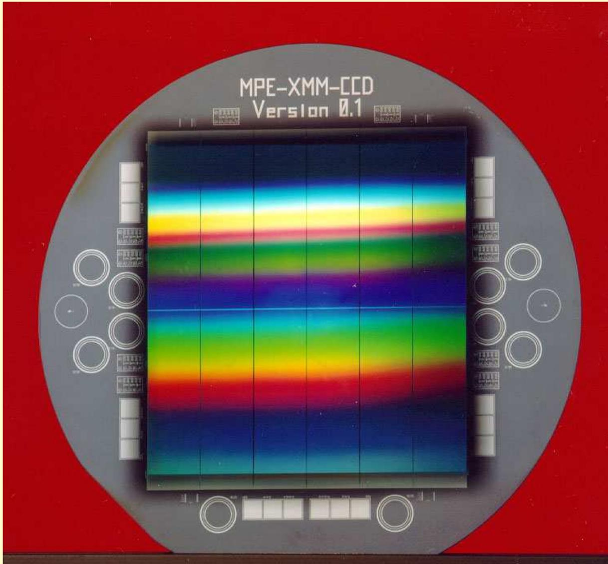
*XMM-Newton*: Array of individual backside illuminated CCDs on one Silicon wafer  $\implies$  requires extreme care during production
