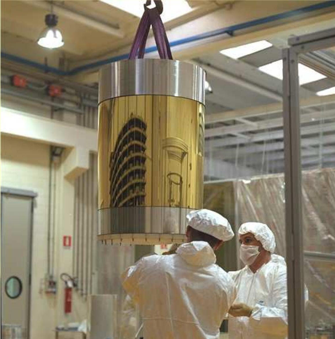
...insertion of Mandrel into electroforming bath
