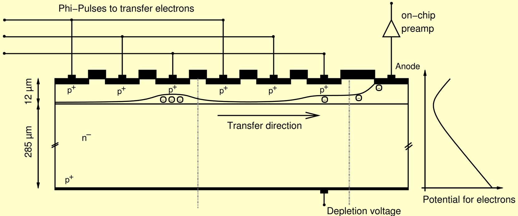
Schematic structure of the *XMM-Newton* EPIC pn CCD.
