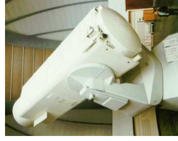
2 m Schmidt telescope at the Landesternwarte Thüringen in Tautenburg near Jena: largest Schmidt telescope in the world.
