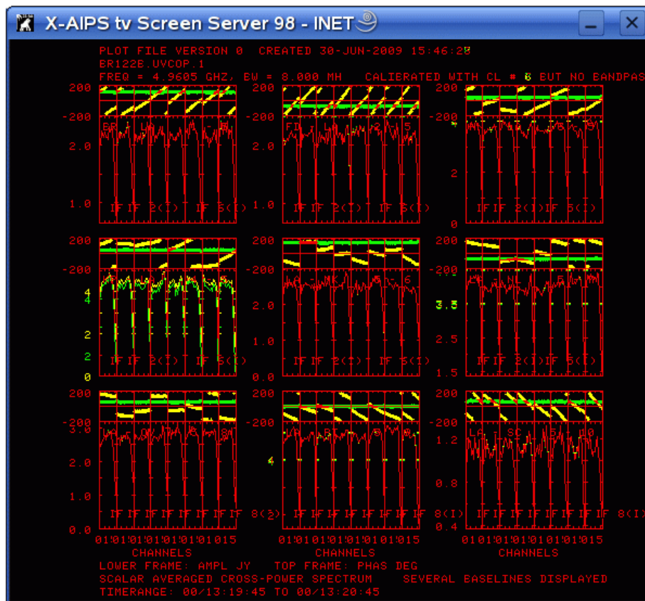
Illustration 9.: Phase and amplitude vs frequency before and after successful phase-cal correction.
