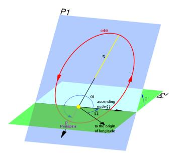
Figure 2: Orbital elements (after http://commons.wikimedia.org/wiki/Image: Orbital\_elements.svg)
