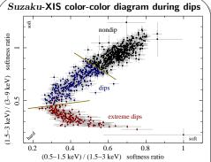
Dipping produces a clear track in this color-color diagram, which was calculated from light curves at 32s resolution. Both colors harden during dips (blue) due to the increased absorption. The final softening (red) of the soft color indicates that the absorber only partially covers the X-ray source.
